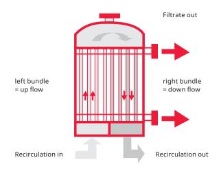
Thanks to this concept, a maximum of packing density and a minimum of pipe connections are achieved. Complete venting and draining is guaranteed by discharging the liquid through the top and bottom plate.
