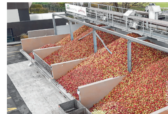
The cider fruit is continually delivered, briefly stored, washed, and fed to the presses. The plant is approx. 80% automated.
